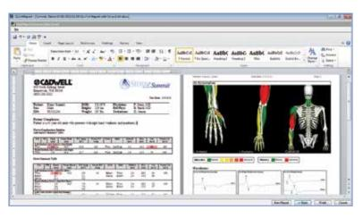
**Autonomic Studies** include RR interval and Sympathetic Skin Response. RR Interval includes automatic or manual calculation of max/min ratio and support for normal and deep breathing, valsalva maneuver, and 30:15 ratio.
