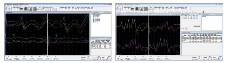
**Evoked Potentials** include somatosensory, auditory, and visual modalities with display and storage of unlimited number of waveforms. Auto-cursors for marking important waveform features with automatic side-to-side comparison and highlighting of abnormal values. Normal or Odd/Even averaging modes. Adjustable artifact rejection and support for third-party stimulators via Trigger In/Out.
