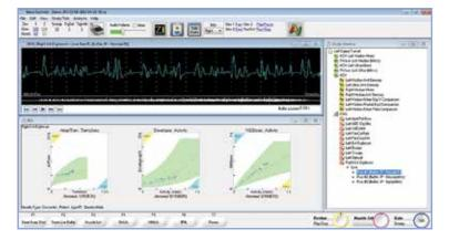
**Multi-MUP Analysis:** Signal decomposition and template matching is used to extract, identify, and sort motor unit action potentials from an epoch of EMG. Typically 1 to 6 motor units can be extracted from one 10 second epoch. Includes flexible editing features and summary display of all acquired MUPs. Can be performed real-time or offline.
