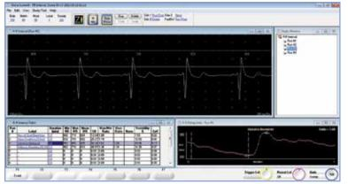
**Advanced Studies** include Macro EMG, MUNE (motor unit number estimation) and multiple stimulus configurations utilizing the two independent electrical stimulators with adjustable train lengths and delays.
