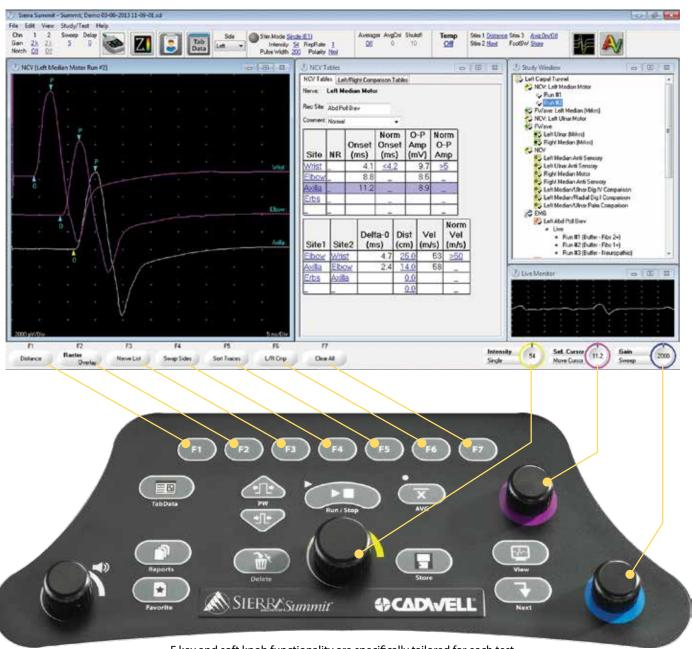
F key and soft knob functionality are specifically tailored for each test protocol to maximize ease of use and facilitate rapid data acquisition
